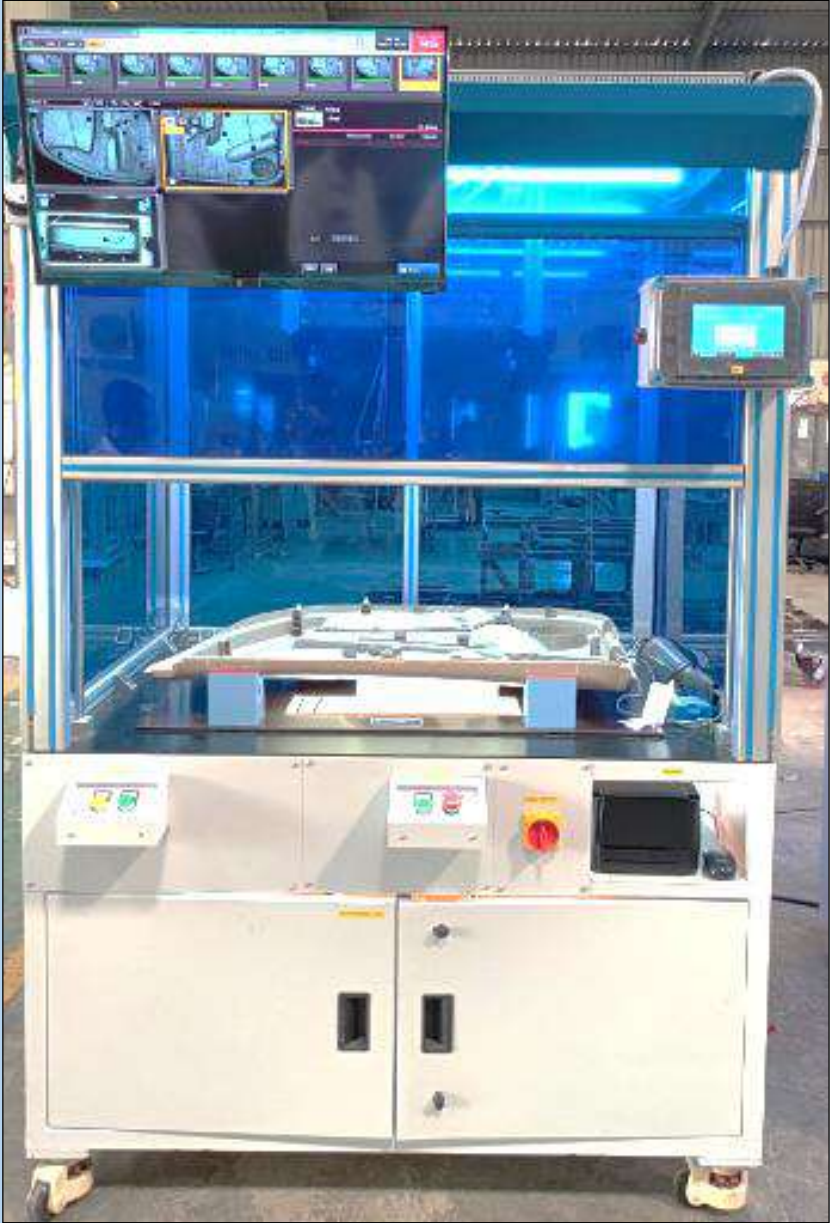
Vision Inspection Station
